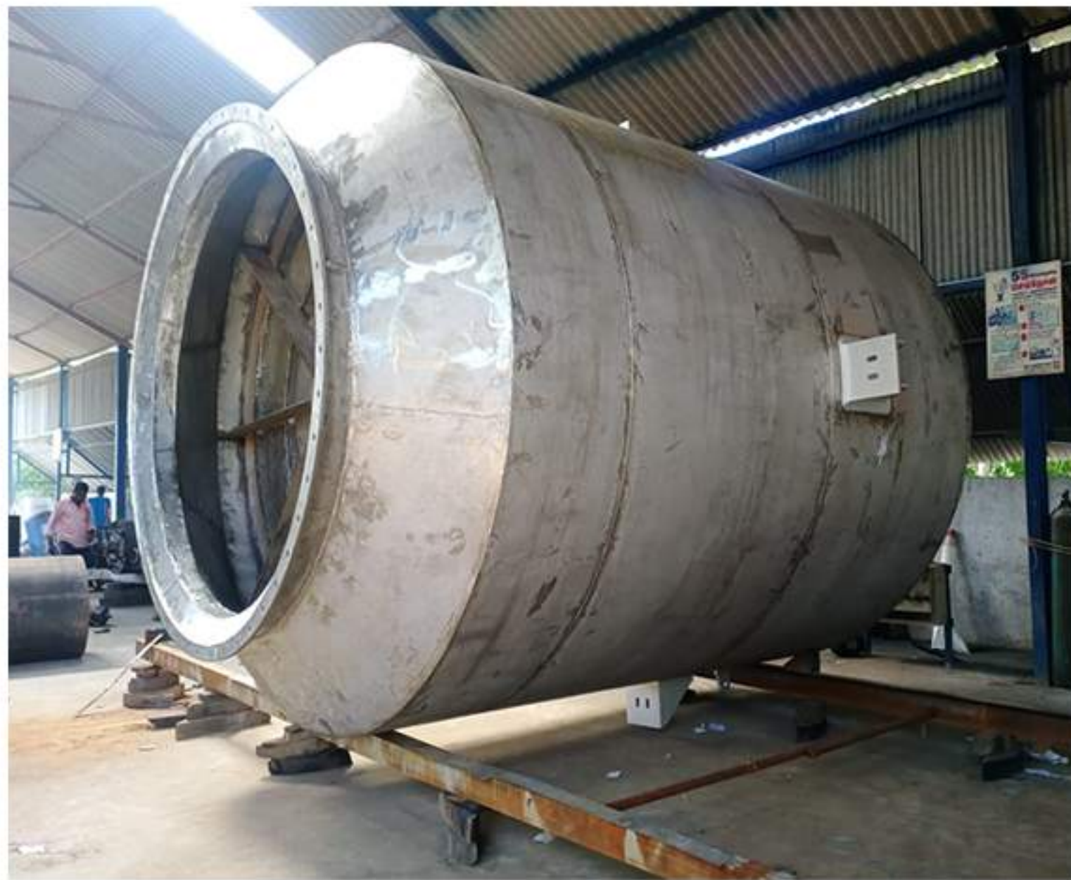
13MW Gas Turbine Silencer
