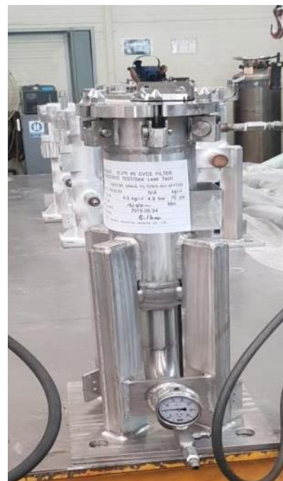
Nuclear Reactor Drain Filter (CVCS Filter)
