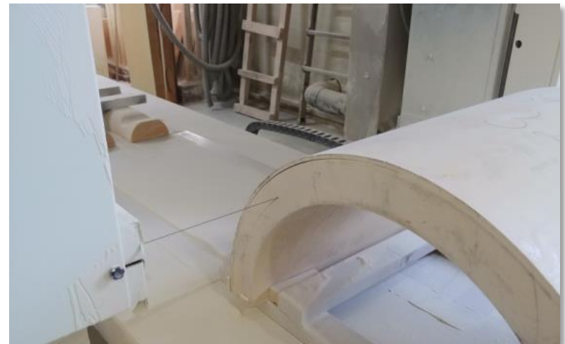
CNC Wire cutting Machining for the Urethane blocks
