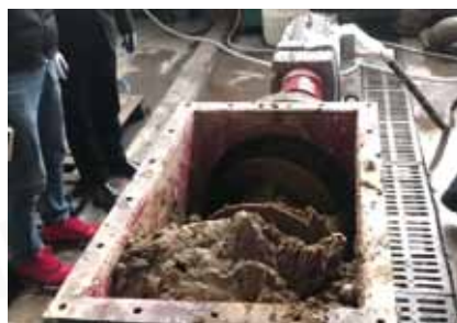
Pump Tested with Mud Cake 28% Solid Content
