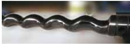
Rotor with vacuum quenching treatment
