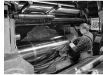
Rubber compounding process
