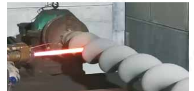
Rotor with spray welding treatment
