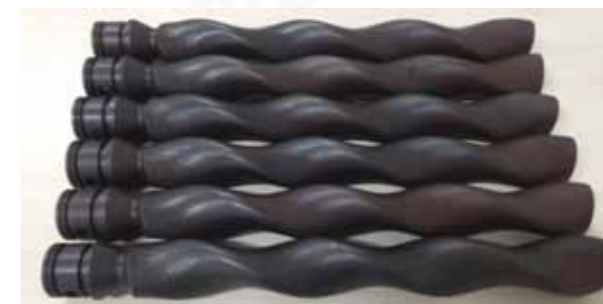
Rotor with vacuum quenching treatment
