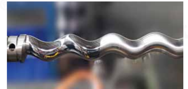
Rotor being mirror-grade polished
