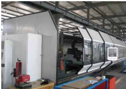
Stator core manufactured field on PS1000 CNC
