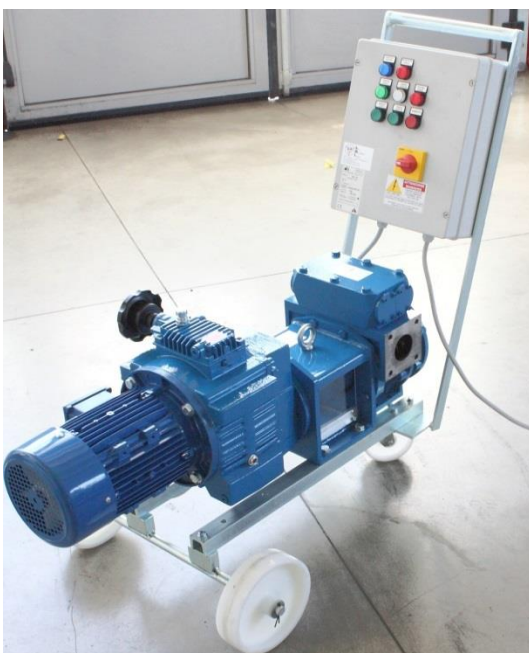
Pump with trolley, panel and speed variator
