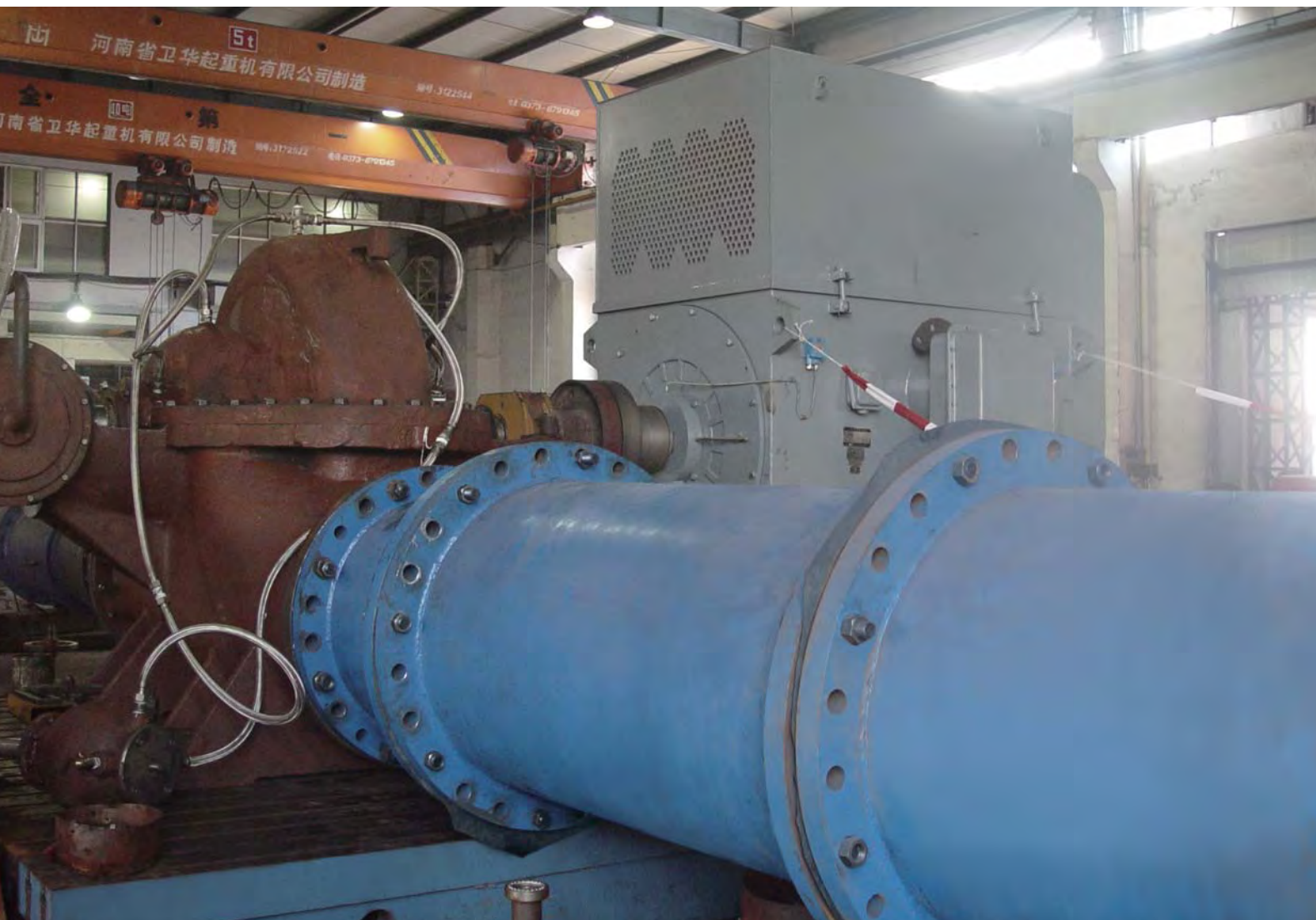
□SLOW1400-1280双吸泵测试现场 SLOW1400-1280 double-suction pump test site
