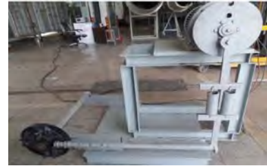
Key slot Fatigue test
