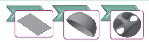
Starting from the metal sheet, the material is pressed and deformed to get the required shape; the parts are welded together and machined with special systems to achieve a perfect body; the result is a very light but high pressure resistance housing. The raw materials come from Europe and we are the only one providing a 100% Italian manufacturing.
