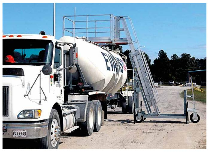
The mobile access cart is designed to provide drivers and operators with a flexible and safe access on to tankers of varying heights, either to sample or load product
