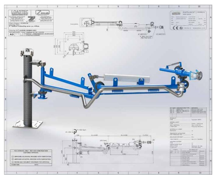
Petroleum/fuel tanker filling via low level connections provides operators with the potential to load multiple compartments simultaneously as well as having automatic high level alarms for each compartment
