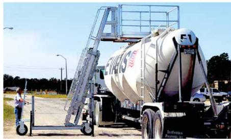
To provide easy mobility the access cart is fitted with 0.4m foam-filled wheels. Levelling jacks at each corner provide a stable and firm base for safe ladder extension. The ladder is extended and retracted using a simple hand winch operation and the cart is easily moved around site using a steering handle with tow bar.
