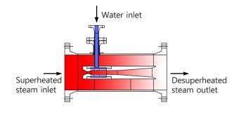
heat which is extracted to evaporate the injection water. This minimizes the time of the suspension of the water particles in the steam so that all the water is evaporated and none falls to the inside walls of the pipe work.
