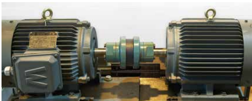
Figure 5: Wear test stand with two misaligned 5 HP motors (controls on each)
