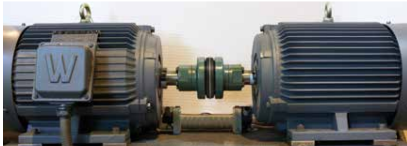
Figure 2: Start-stop fatigue test stand with two aligned 15 HP motors
